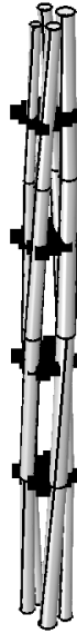
Figure 2.31. Nerve model with rotating fascicles to with four plates with 16 Point Sources electrodes each.
